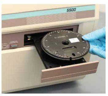
The Harshaw 5500 is offered with a variety of carrier disks, designed to handle a wide range of material, in a number of different formats (ribbons, chips, rods, and micro-cubes) and sizes, allowing you to choose the approach that best suits your application.
