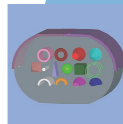
Shapes phantom Customise with 14 internal VOIs, outer bolus/mask that can be moved, deleted, re-sized, density filled.
