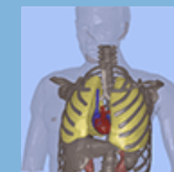
Thorax phantom Lungs & heart can be moved, inflated, deflated. 4D phase CT series created from user/RPM imported signal.
