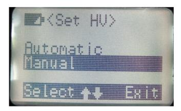
Use the left and right arrows to move the cursor to the correct position and then use the up and down arrows to set the voltage to 300V. make sure that the setting is saved when exiting the menu. If in doubt repeat procedure to check that 300V is now set.
