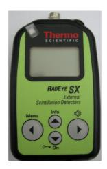
The RadEye is unmodified and retains the same keypad controls and options as the real instrument.
