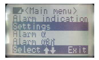
Use the up/down button to scroll through Settings to Set HV, press the menu button to select.
