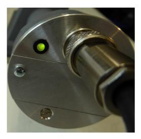
It should be noted that the STS electronics draw a significant current whilst sensing and so although the battery icon may suggest the batteries are ok please change them before any other action is taken. The DP6 requires 4 AA cell batteries.
